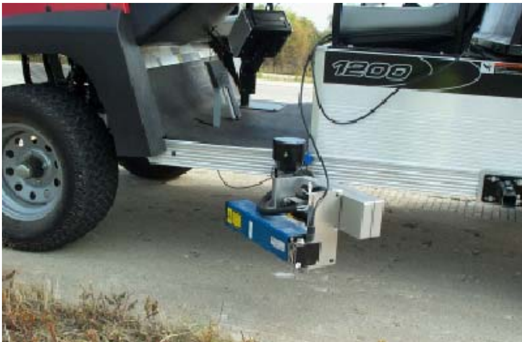
Figure C.4. SSI lightweight inertial profiler, sensor arrangement.
