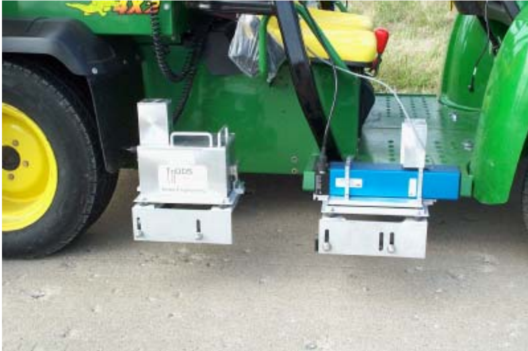
Figure C.5. Ames Engineering lightweight inertial profiler, sensor arrangement.
