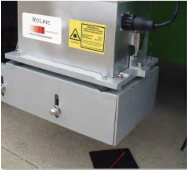
Multipoint laser systems like the RoLine sensor deliver more accurate readings on textured surfaces.
